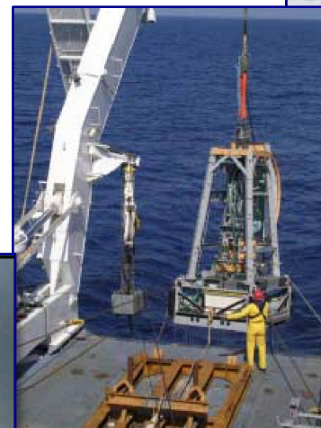
In Situ geotechnical measurements (IFREMER Penfeld Penetrometer)
