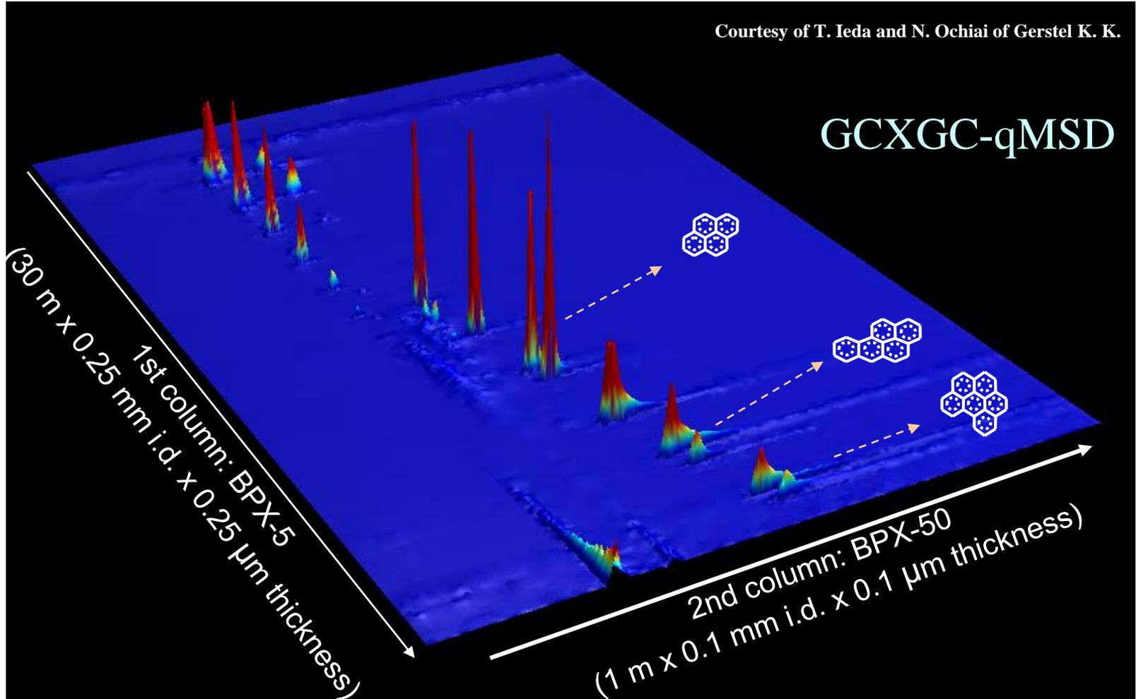
1<sup>st</sup> column: BPX-5 (30 m x 0.25 mm i.d. x 0.25 μm thickness)
