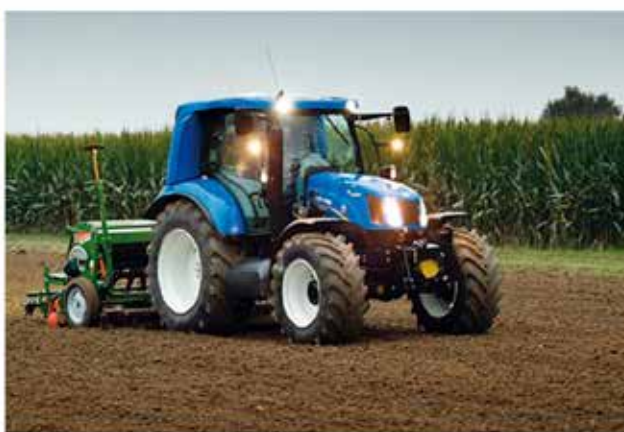
New Hollande T6.140 Biomethane powered tractor
