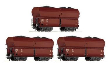
Both trucks that the wagons are specially shaped to easily download the solid fuel by lift and tilt of the body itself by the hydraulic pistons or opening of the side doors of the body.
