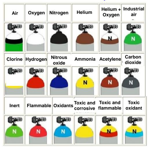
Air: white + black, oxygen: white, nitrogen: black, helium: brown, helium + oxygen: white + brown + N, industrial air: light green + N, chlorine: yellow, hydrogen: fire red, nitrous oxide, purple, ammonia: yellow + N, acetylene: brown + N, carbon dioxide. dark gray + N, inert very light green + N, flammable: red + N, oxidants: light blue + N, toxic and corrosive: yellow, toxic and flammable: fire red + yellow + N, +
