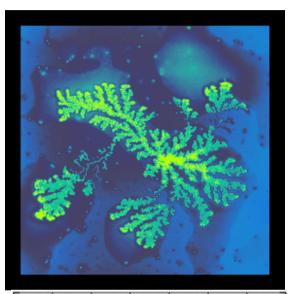
REAL IMAGE (by Atomic Field Microscopy) of a gold colloid of about 15 nm on a mica substrate
