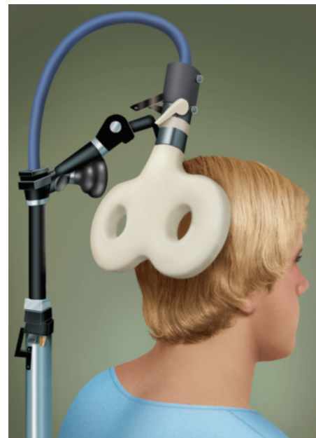
Figure 8.26 TMS coil positioned to present a magnetic field to the back of the person's head.
