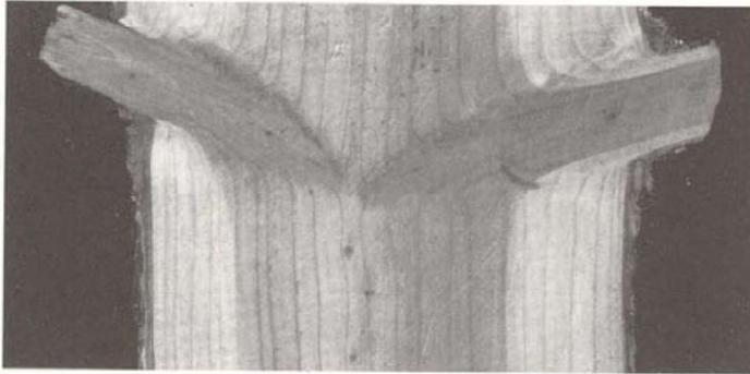
Sawn timber beam with knots
