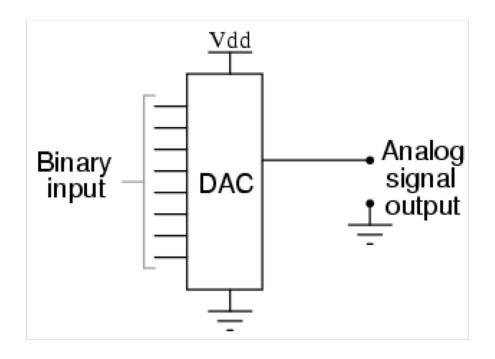
An actuator is commonly driven by a voltage that may be converted from a number by a DAC. An actuator that is packaged with a DAC is called a **digital actuator**.
