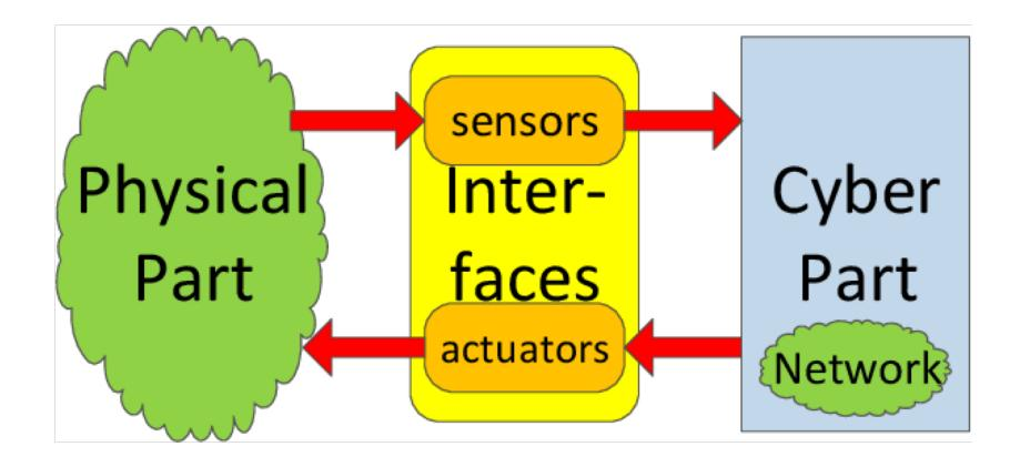
**Sensor**: a device that **measures** a physical quantity
