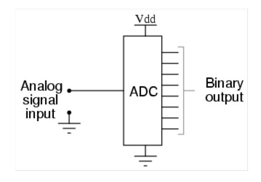
A sensor that is packaged with an ADC is called a **digital sensor**, whereas a sensor without an ADC is called an **analog sensor**
