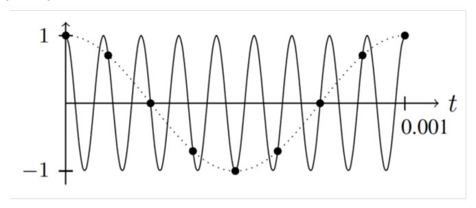
Careful modeling of the signal sources and analog signal conditioning or digital oversampling are necessary to counter the effect.
