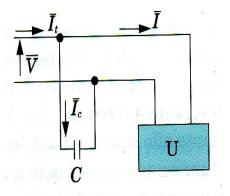
Putting in parallel a capacitor which absorbs a current  $I_c$  anticipated of 90° in comparison to the voltage, it is possible to obtain the total current given by the vector sum:
