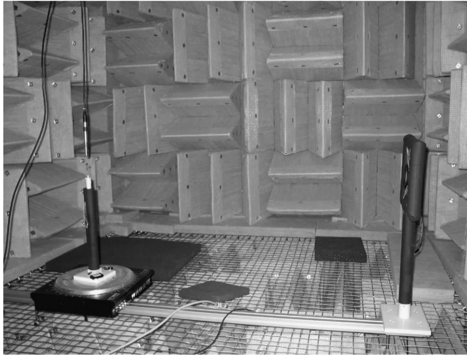
Figure 3.17 Setup in an anechoic chamber for measurement of a microphone's directivity
