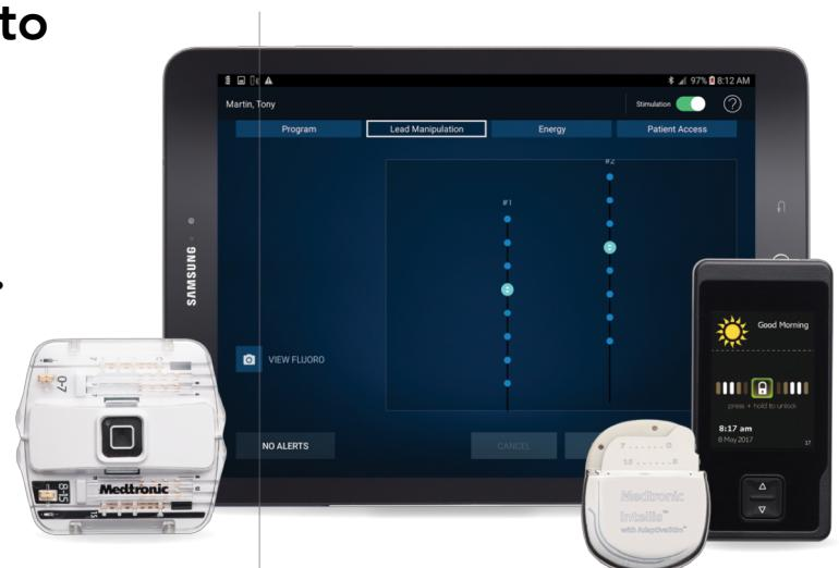
Medtronic implantable device for treating chronic pain by delivering neurostimulation at the spinal cord is connected to a Samsung Galaxy Tab S2, to allow data capturing and IPG controlling
