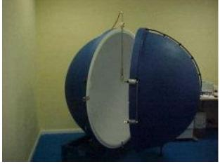
The measure is carried out by means of a photovoltaic cell placed behind a small slit practiced on the surface of the sphere. To avoid that the cell directly receives the luminous rays emitted from the source, between the two is placed a diffusing screen. A.A. 2018-2019
