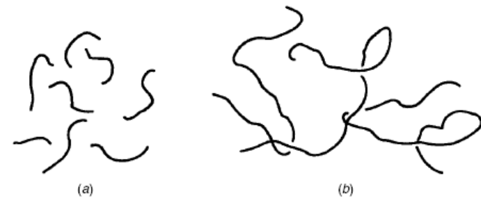
Figure 1.3 Entanglement of polymer chains. (a) Low molecular weight, no entanglement. (b) High molecular weight, chains are entangled. The transition between the two is often at about 600 backbone chain atoms.
