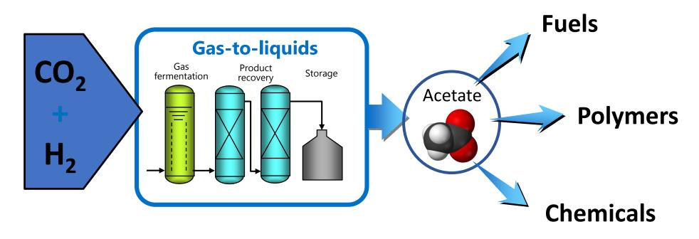
**CO<sub>2</sub> uptake and capture** demonstrated in a <u>continuous</u> fermentation
