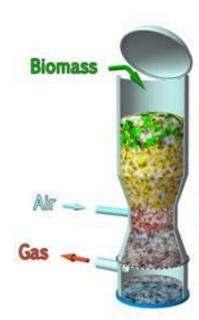
Drying Zone Pyrolysis Zone Combustion Zone Reduction Zone Ash Removal
