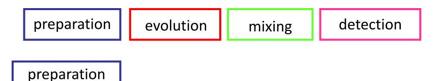
During preparation, the spin system is prepared in a non equilibrium coherent state, which is going to evolve during the following stages. In the simplest experiments (e.g. COSY) the preparation is a single pulse
