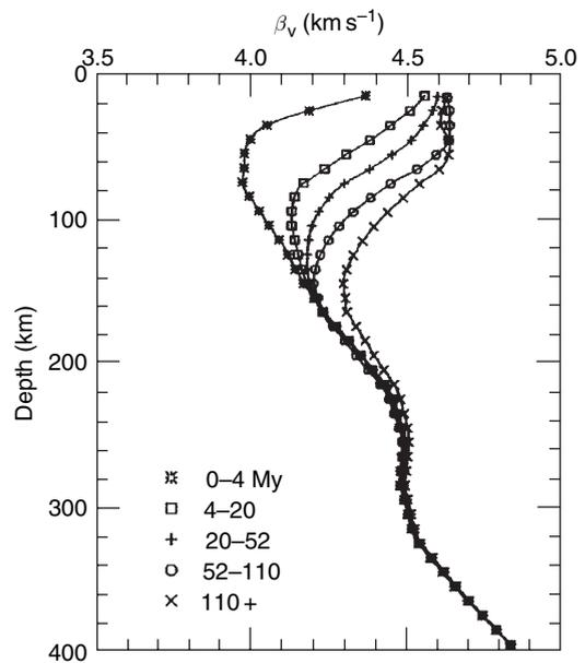
**Figure 4** Vertically polarized shear-wave velocity in the Pacific as a function of depth in various age intervals determined from Rayleigh wave dispersion (Nishimura and Forsyth, 1989). Note that shear-wave velocity changes with age at depths greater than would be consistent with a plate model that fits the depth–age relationship ( $\leq 125$  km). Changes with age continue beneath seafloor with ages exceeding 110 My.
