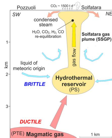
**Fig. 4.** Conceptual model of the hydrothermal system feeding the Solfatara fumaroles. PTE and pressurized spheroid (PS) refer to the sources of the ground deformation that is active at Cfc, according to Amoroso et al. (2014a, 2014b).
