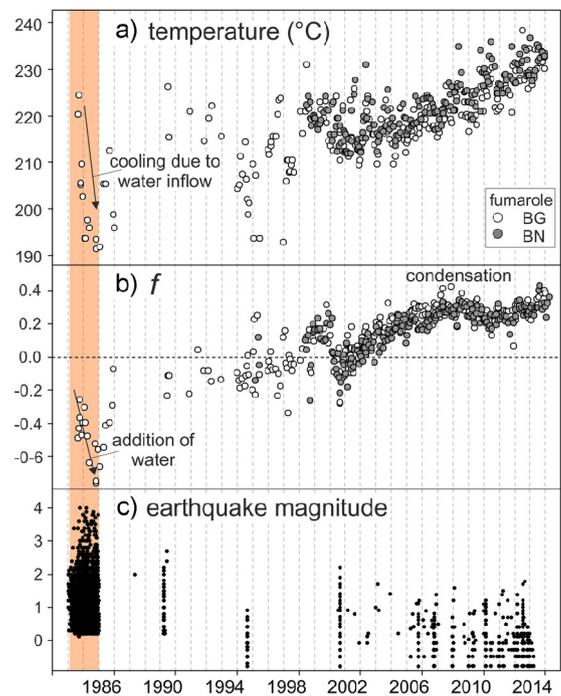
Fig. 7. Temperature (a) and  $f$  values (b) inferred from thermodynamic computations within the H<sub>2</sub>O–H<sub>2</sub>–CO<sub>2</sub>–CO gas system. The variable  $f$  refers to the fraction of the water removed (sign +) or added (sign –) during the transfer of the gas from the equilibration zone to the fumarole. Earthquake magnitudes are reported for comparison in (c) (data from D’Auria et al., 2011).
