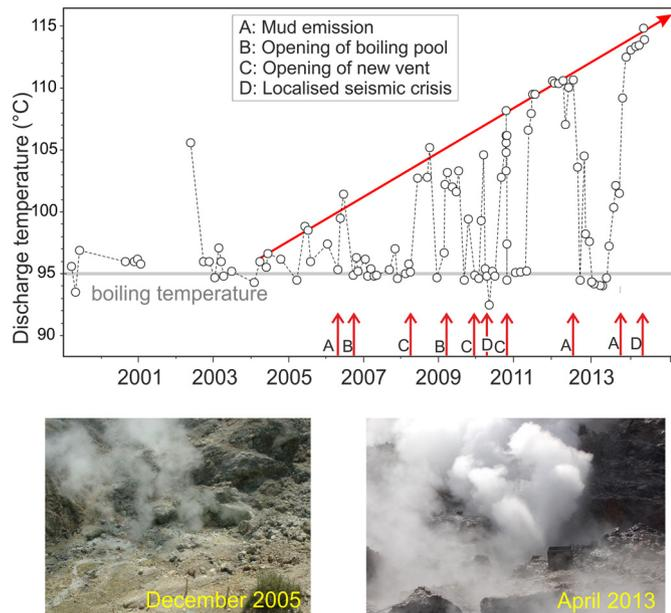
**Fig. 2.** Time series of discharge temperatures at Pisciarelli fumarole, and chronogram of localized phenomena that have affected the hydrothermal site (red arrow). The two pictures highlight the strong increase in fumarolic flow rate from 2005 to 2013. (For interpretation of the references to color in this figure legend, the reader is referred to the web version of this article.)
