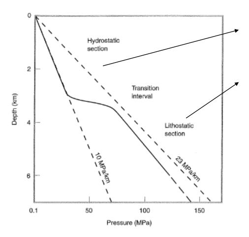
HYDROSTATIC pore pressure weight of the overlying fluid
