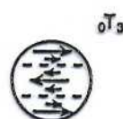
FIGURE 4.24 (Top) Surface and radial patterns of motions of spheroidal modes. (Bottom) Purely radial modes involve no nodal patterns on the surface, but overtones have nodal surfaces at depth. Toroidal modes involve purely horizontal twisting of the Earth. Toroidal overtones ( {}_1T_2 ) have nodal surfaces at constant radii across which the sense of twisting reverses. (After Bolt, 1982.)
