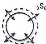
FIGURE 4.24 (Top) Surface and radial patterns of motions of spheroidal modes. (Bottom) Purely radial modes involve no nodal patterns on the surface, but overtones have nodal surfaces at depth. Toroidal modes involve purely horizontal twisting of the Earth. Toroidal overtones ( {}_1T_2 ) have nodal surfaces at constant radii across which the sense of twisting reverses. (After Bolt, 1982.)
