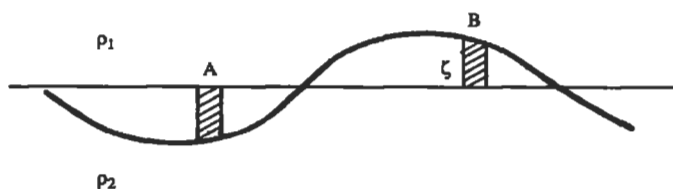
Figure 7.28 Calculation of potential energy of a two-layer fluid. The work done in transferring element A to B equals the weight of A times the vertical displacement of its center of gravity.
