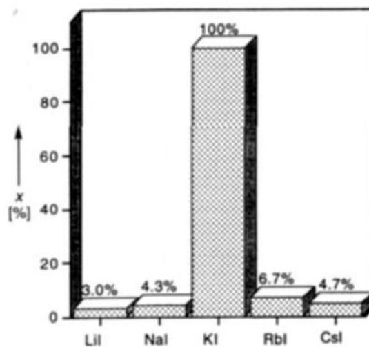
Figure 3. Uptake of alkali metal ions by **3** after treating its chloroform-methanol solution (4/1,  $[3] = 1 \text{ mM}$ ) with 10 equivalents of alkali metal iodide. The complexation ratio  $x$  was determined by integration of the  $^1\text{H}$  NMR spectra after the samples had been left to stand for 90 h. In the case of KI, equilibrium was reached within an hour.
