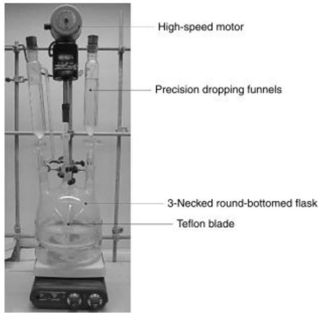
Figure 2.1 Typical apparatus used for high-dilution synthesis.
