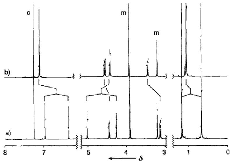
Figure 2.  $^1\text{H}$  NMR spectrum of **3** [500 MHz,  $\text{CDCl}_3/\text{CD}_3\text{OD}$  4/1 (v/v)]: a) pure, b) with 10 equivalents of solid potassium iodide (c, m: solvent peaks corresponding to chloroform and methanol, respectively).
