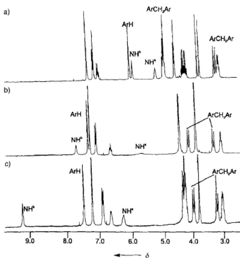
Fig. 1. <sup>1</sup>H NMR spectra of **2** (CDCl<sub>3</sub>, 5 mM). a) Uncomplexed, b) [2·Na]ClO<sub>4</sub>, c) [2·NaCl]. For NH<sup>a</sup> and NH<sup>b</sup> see Scheme 1; for ArH and ArCH<sub>2</sub>Ar see the text or ref. [14].
