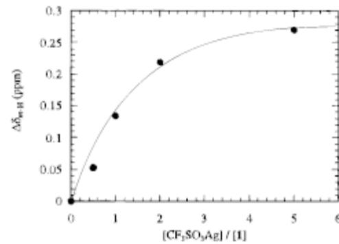
**Figure 7.** Chemical shift change in  $\delta_{m-\text{H}}$  of  $\text{IH}^+$  induced by added  $\text{CF}_3\text{SO}_3\text{Ag}$ : 30 °C,  $[\text{I}] = 5.00 \text{ mM}$ ,  $[\text{TFA-}d] = 600 \text{ mM}$ ,  $\text{CD}_2\text{Cl}_2:\text{CD}_3\text{OD} = 4:1 \text{ v/v}$ .
