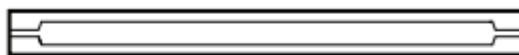
Figure 6: Thermo Scientific liner for TRACE 1300/1310 and Agilent Split/Splitless inlet, Double Taper 4 x 78.5 mm internal dimension (P/N 453A1355)
