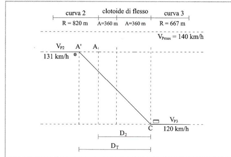
$$D_{T2} = \frac{V_{p,2}^2 - V_{p,3}^2}{3,6^2 \cdot 2 \cdot a} = \frac{131^2 - 120^2}{3,6^2 \cdot 2 \cdot 0,8} = 133,15 \quad [\text{m}]$$
