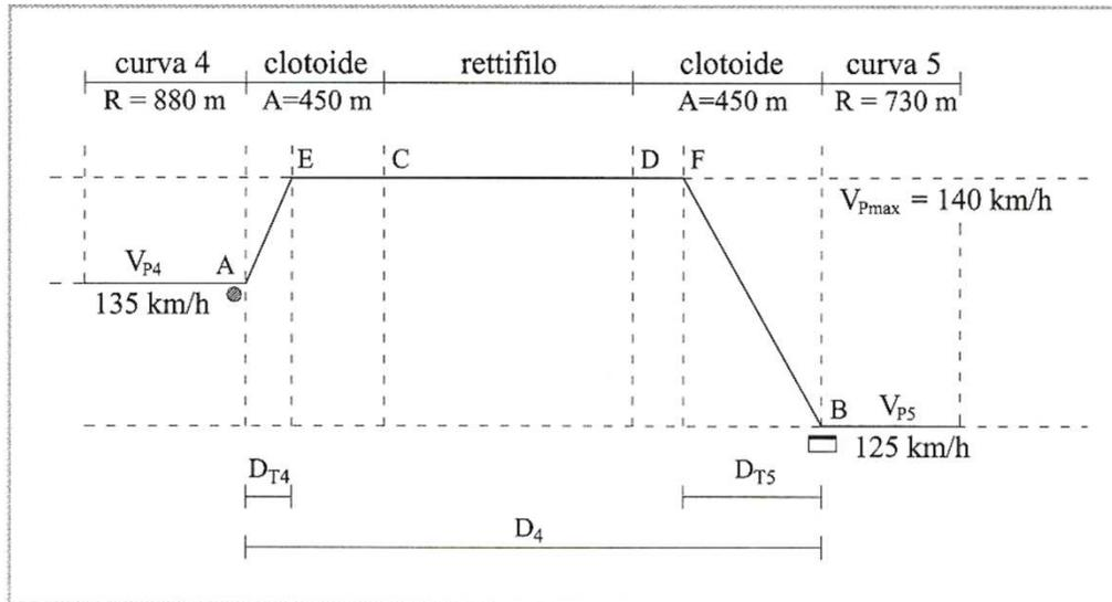
$$D_{T,4} = \frac{V_{p,max}^2 - V_{p,4}^2}{3,6^2 \cdot 2 \cdot a} = 66,31$$
