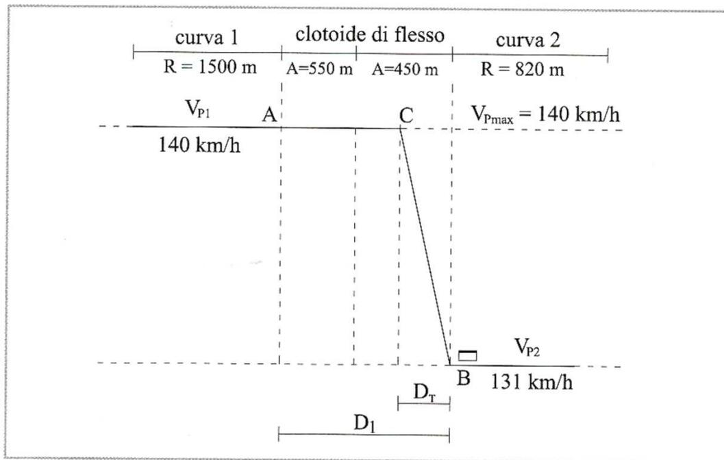
$$D_{T1} = \frac{V_{p,1}^2 - V_{p,2}^2}{3,6^2 \cdot 2 \cdot a} = \frac{140^2 - 131^2}{3,6^2 \cdot 2 \cdot 0,8} = 117,62 \quad [\text{m}]$$
