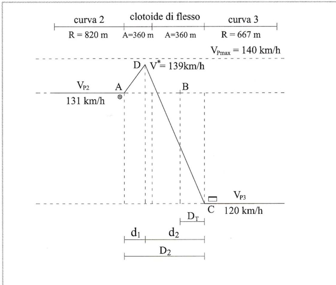
$$\left\{ \begin{array}{l} V_p^{*2} = V_{p2}^2 + 2 a d_1 \\ V_{p,3}^2 = V_p^{*2} - 2 a d_2 \\ D_2 = d_1 + d_2 \end{array} \right.$$
