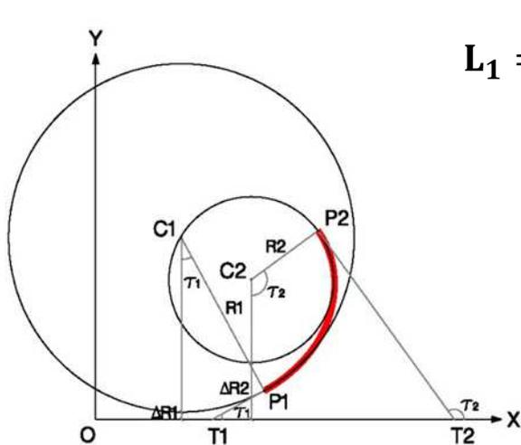
$$L_1 = \frac{A^2}{R_1} \quad L_2 = \frac{A^2}{R_2}$$
