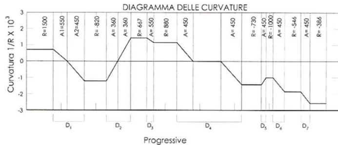
$$D_T = \frac{V_{p,1}^2 - V_{p,2}^2}{3,6^2 \cdot 2 \cdot a} = \frac{\Delta V \times V_m}{12,96 \cdot a}$$
