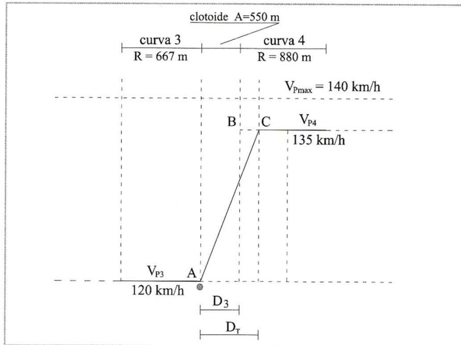
$$D_{T3} = \frac{V_{p,4}^2 - V_{p,3}^2}{3,6^2 \cdot 2 \cdot a} = 184,46$$
