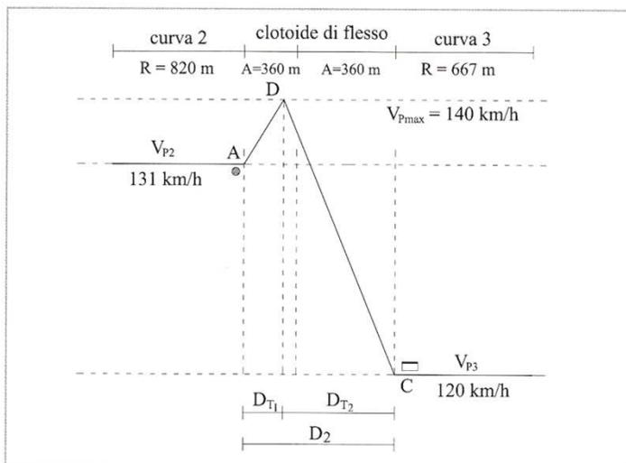
$$D_{T2} = \frac{V_{p,2}^2 - V_{p,3}^2}{3,6^2 \cdot 2 \cdot a} = 133,15$$
