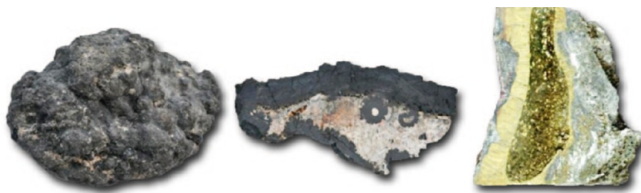
Fig 2: Three types of mineral resources of the deep sea. From left to right: A poly-metallic nodule, an example of manganese crust and a chimney with hydrothermal sulphides (from [2]).
