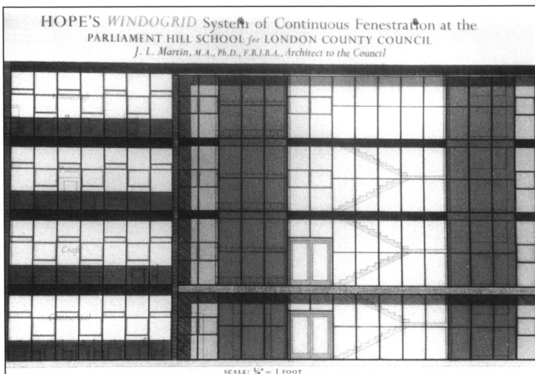
Fig. 14 The Windowgrid system in use at Parliament Hill School, London (from Henry Hope and Sons Ltd., Hope's Window Walls , 1956).
