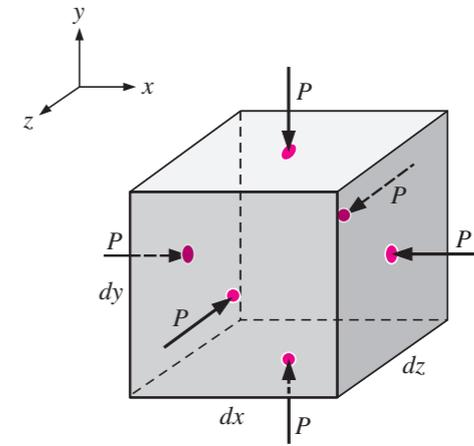
Hydrostatic pressure is the same as the thermodynamic pressure from study of thermodynamics.  $P$  is related to temperature and density through some type of equation of state (e.g., the ideal gas law).
