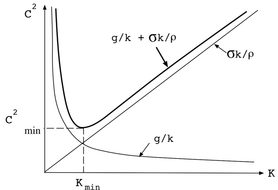
and the  $k_{\min} = (\rho g/\sigma)^{1/2}$ , associated to a wavelength of 1.73 cm for the water, corresponds to a minimum for phase velocity (23.2 cm/s).
