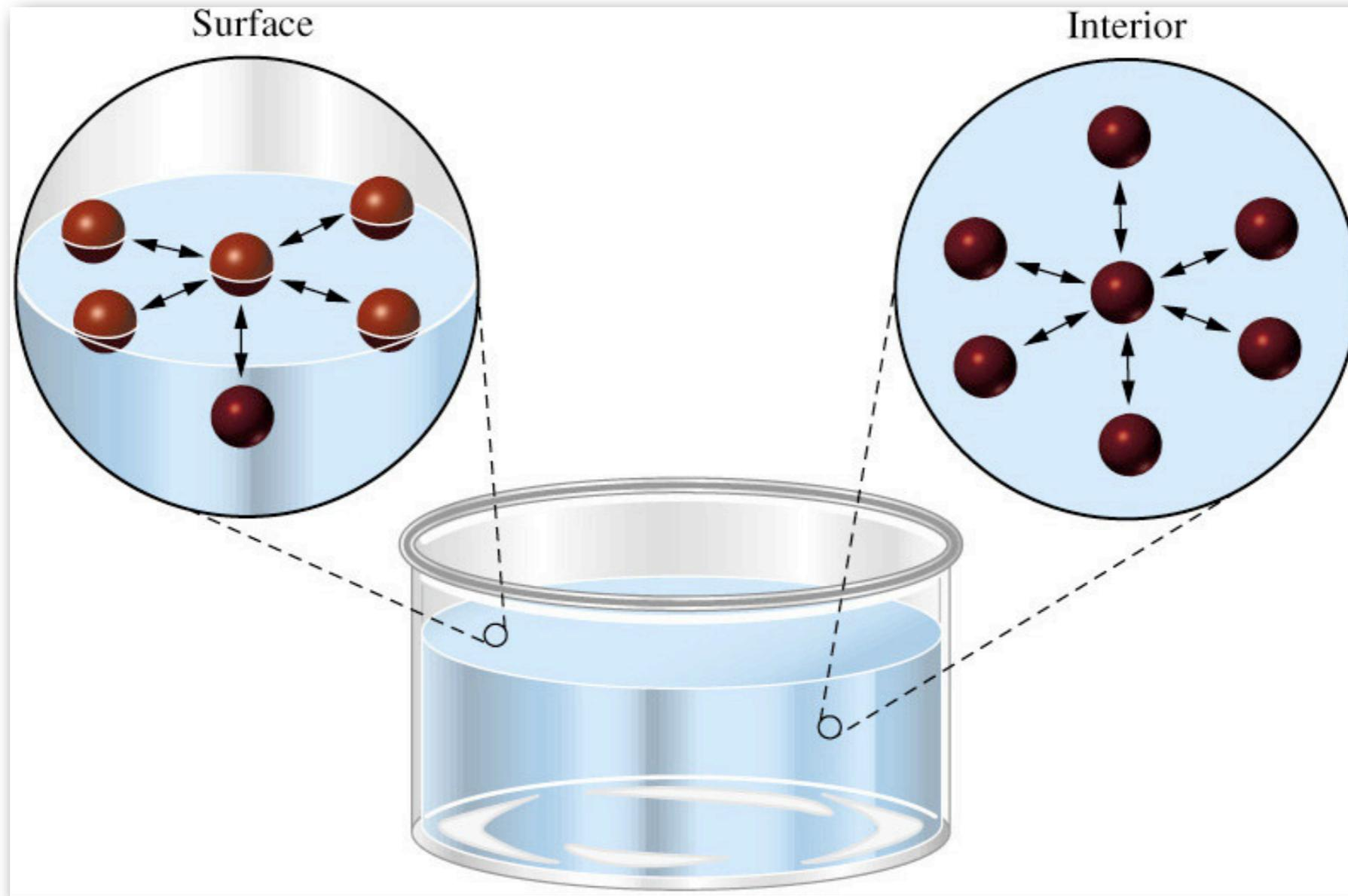
Molecules have a tendency to be drawn into the interior of a liquid to the greatest extent possible, leaving a minimum of surface area.
