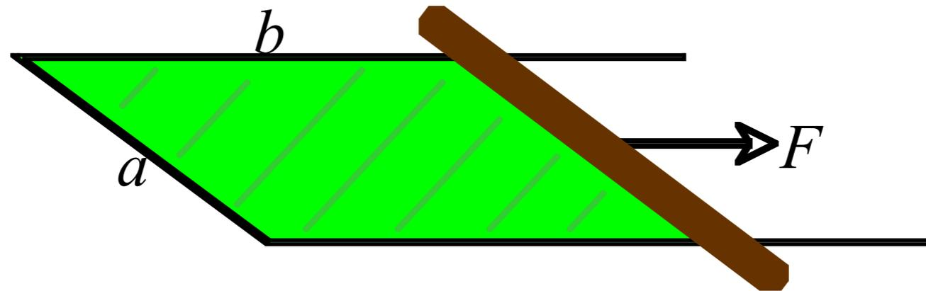
The work done to pull a thin film of fluid has to be equal to the increase in energy:
