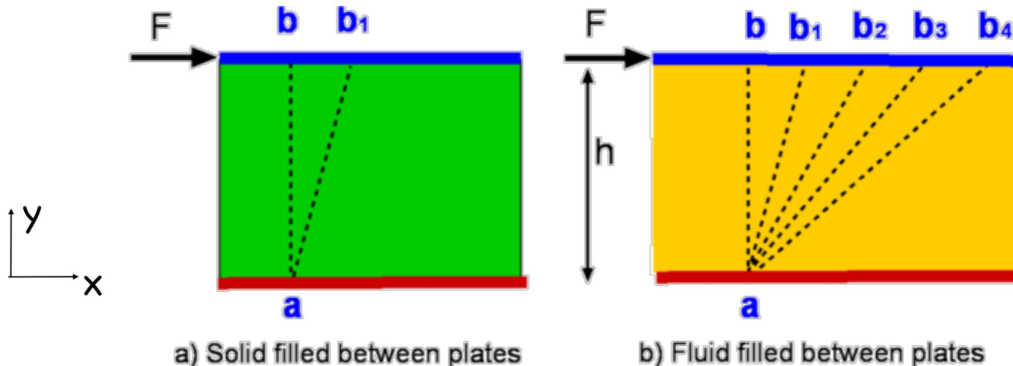
Fluids are qualitatively different from solids in their response to a shear stress. Ordinary fluids such as air and water have no intrinsic configuration, and hence fluids **do not develop a restoring force** that can provide a static balance to a shear stress. When the shear stress is held steady, and assuming that the geometry does not interfere, the **shear deformation rate**, may also be steady or have a meaningful time-average.
