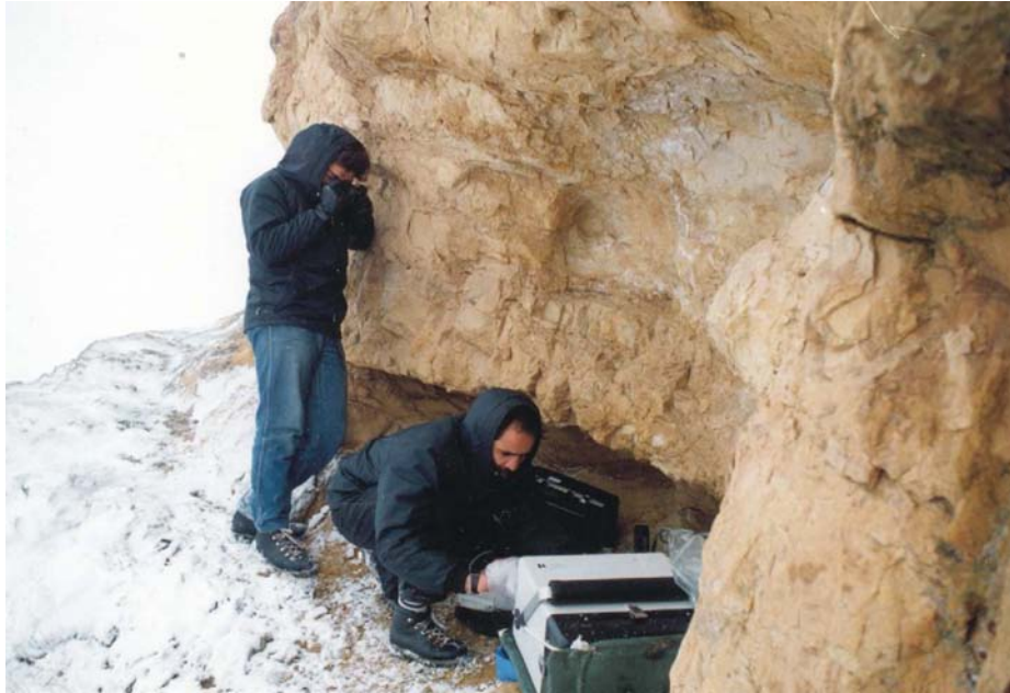
Fig. 7.14 Hiding with the noise recording equipment on a windy day with snowfall in a small cave on the lee-side of a rock cliff. Surface recordings under adverse weather conditions of the noise level at this site in NW Iran were close to the best sites in good weather.
