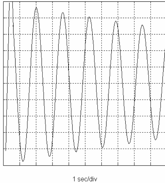
Figure 2a Seismometer step response: open circuit.
