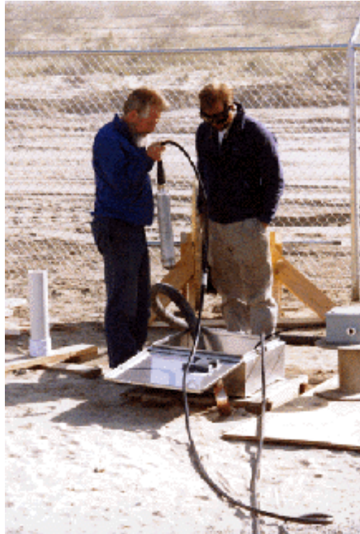
Fig. 7.64 Lowering a borehole accelerometer into the cased borehole.
