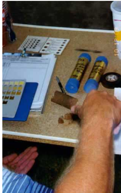
Fig. 7.68 Drive samples being collected for later laboratory testing.
