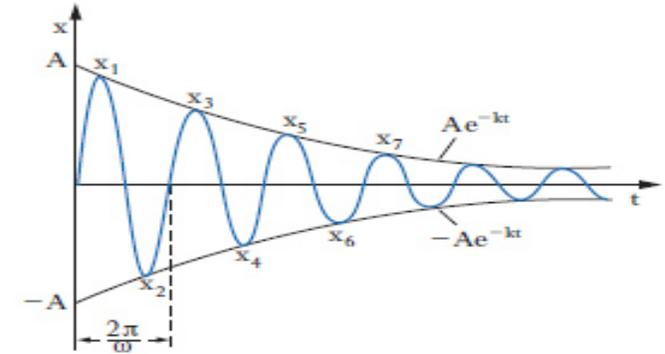
$$x_{eq} = \frac{1}{2} \left[ \frac{1}{3} (x_1 + x_3 + x_5) + \frac{1}{2} (x_2 + x_4) \right] \quad \text{con } \Delta x_{eq} = 0.5 \text{ div}$$
