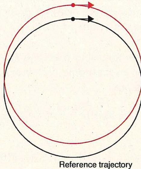
In a uniform magnetic field, the trajectories of two particles with some small initial offset will “oscillate” around each other.
