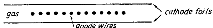
Fig. 19 Multi-wire chamber. Typically, the distance between the cathode foils is 10 mm, the distance between wires 1 mm, their diameter 5 to 50 \mu\text{m} and their potential + 5 kV.
