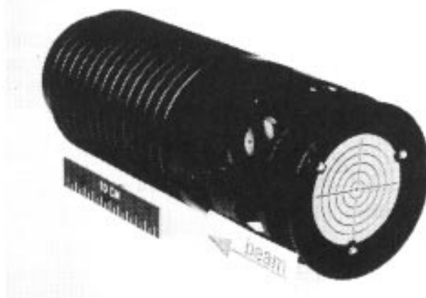
Fig. 25 Scintillator plate mounted on the antiproton production target of the CERN Antiproton Accumulator.
