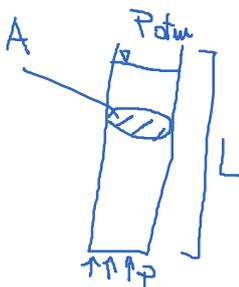
$$\begin{aligned} p \cdot A &= p_{\text{atm}} \cdot A + \rho_{\text{olio}} \cdot V_{\text{olio}} \cdot g \\ &= p_{\text{atm}} \cdot A + \rho_{\text{olio}} \cdot (A \cdot L) \cdot g \\ p &= p_{\text{atm}} + \rho_{\text{olio}} \cdot g \cdot L \quad (\text{legge di Stevino}) \end{aligned}$$
