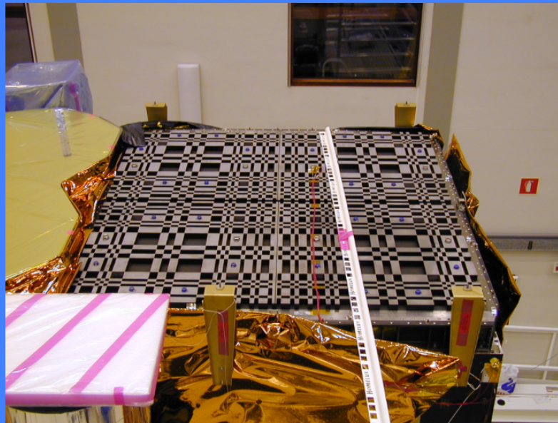
Mask of IBIS (15 keV – 10 MeV) onboard INTEGRAL
