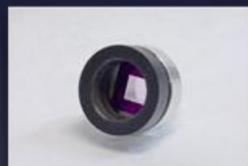
5x5 mm 2 Si 3 N 4 , 100 nm thick membrane at 5° incidence angle
