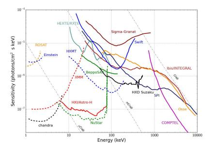
Fig. 21 Three sigma sensitivity, for an exposure time  $T = 10^5$  s and a bandwidth  $\Delta E = E/2$ , of the most relevant missions in the hard X-ray/soft gamma-ray band. Adapted from Virgilli et al. (2017).
