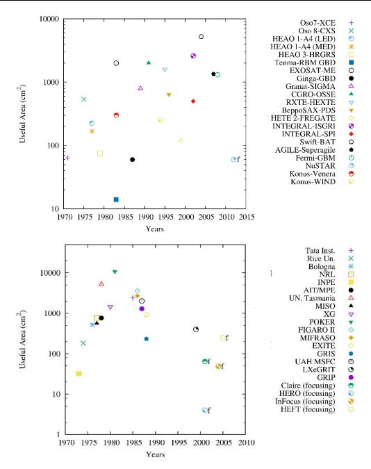
Fig. 20 Trend with time of the useful area, defined as the geometrical area through the collimator or coded mask, of the hard X-ray non-focusing instruments. In the case of focusing instruments (marked with "f"), it is shown the trend with time of the effective area. *Top panel*: Satellite instruments. Data are taken from Table 1. *Bottom panel*: balloon instruments. Data are taken from Table 2.
