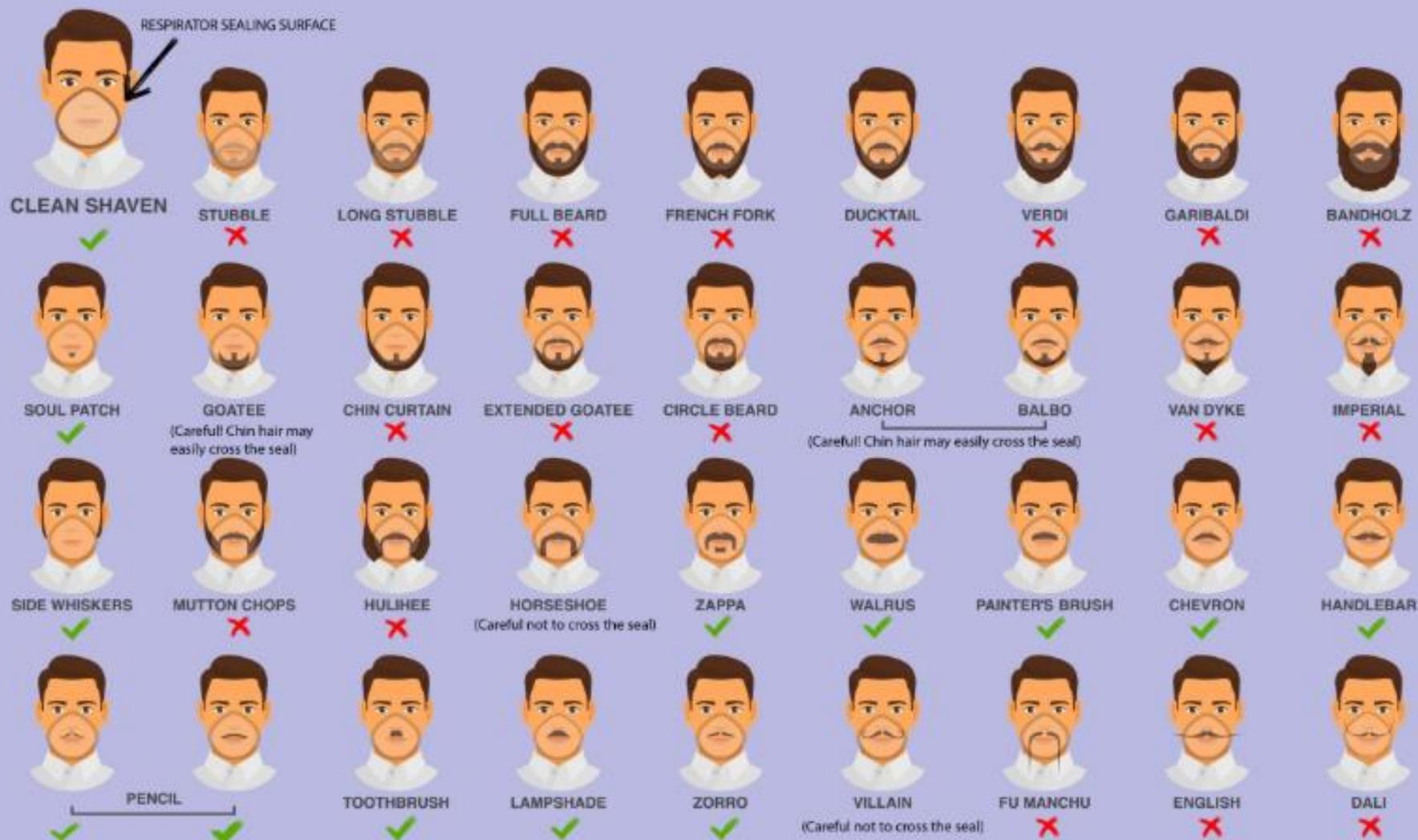
\*If your respirator has an exhalation valve, some of these styles may interfere with the valve working properly if the facial hair comes in contact with it.
