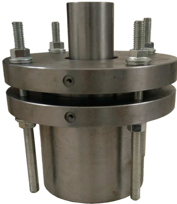
Figure 14.1 - New experimental prototype for the dynamic characterization of the pillar isolator
