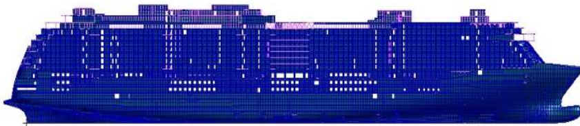
Figure 7.1 - FE model of the cruise ship used for load evaluation
