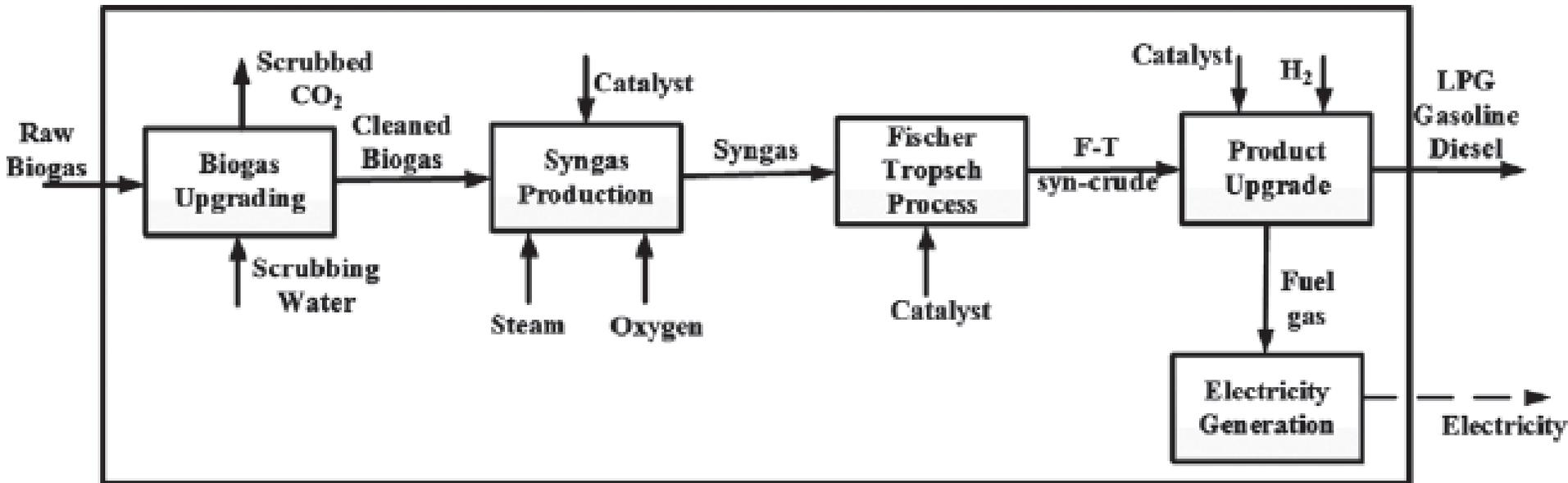
Figure 1. A schematic of a biogas to liquid fuels production technology.
