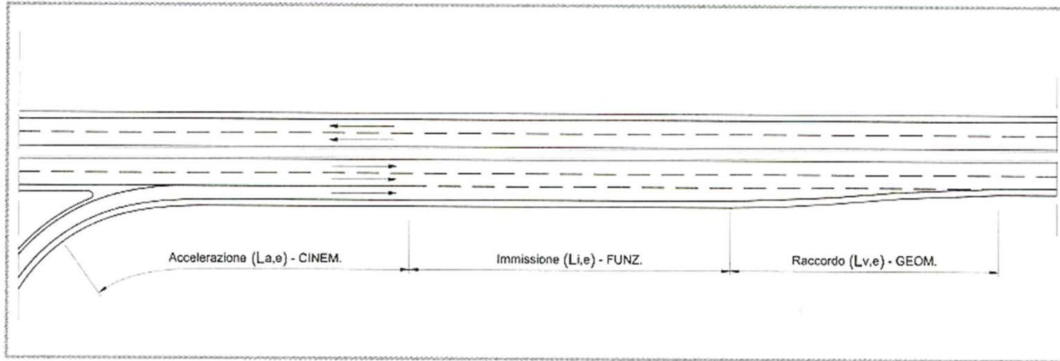
$$L_{a,e} = \frac{v_1^2 - v_2^2}{2a}$$
