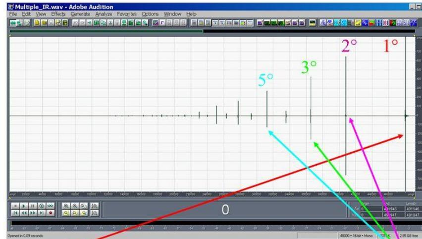
The last impulse response is the linear one, the preceding are the harmonics distortion products of various orders
