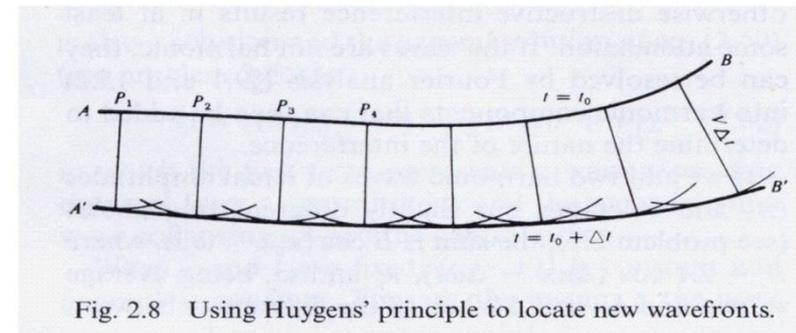
Fig. 2.8 Using Huygens' principle to locate new wavefronts.
