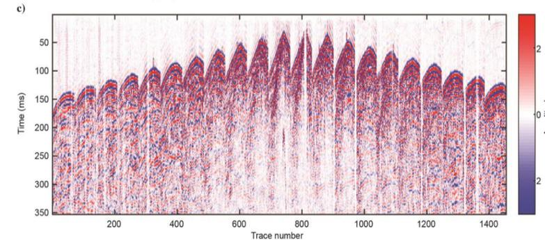
**Figure 5.** (a) Three-dimensional seismic survey and the corresponding fold map for the seismic data collected over Kevitsa Ni-Cu-PGE orebody, northern Finland (after Malehmir et al., 2012), (b) location of a shot and the corresponding recording patch within the acquisition area, and (c) the corresponding pre-processed seismic data (Zirarov et al., 2015) cut to 350 ms.
