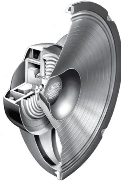
FIGURE 2.2 Loudspeaker incorporating a whizzer cone.
