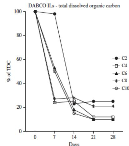
**Fig. 6.** Percentage of total dissolved organic carbon (TDC) calculated for DABCO ILs with different lateral chain length (C2-C10). Results are expressed as % of each DABCO point of the curve set at 100% (Fig. 4). Observations were performed at 0, 7, 14, 21, and 28 days from the inoculums. Experiments were carried out in triplicate, levels were reported as average data ( $n=3$ ).
