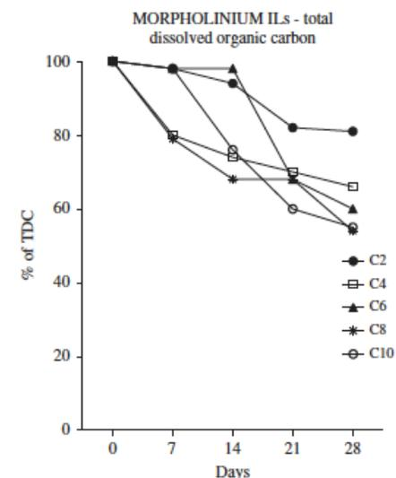
**Fig. 7.** Percentage of total dissolved organic carbon (TDC) calculated for morpholinium ILs with different lateral chain length (C2-C10). Observations were performed at 0, 7, 14, 21, and 28 days from the inoculums. Experiments were carried out in triplicate, levels were reported as average data ( $n=3$ ).
