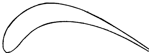
Primary turbine blade section, \theta_c = 110^\circ , t/c = 15 percent
