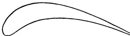
Primary turbine blade section, \theta_c = 95^\circ , t/c = 15 percent
