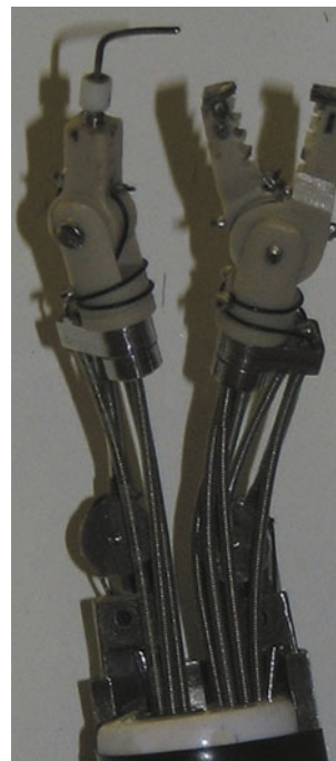
Fig. 4 MASTER. The robotic slave manipulator adapted to the endoscope, Nanyang Technological University
