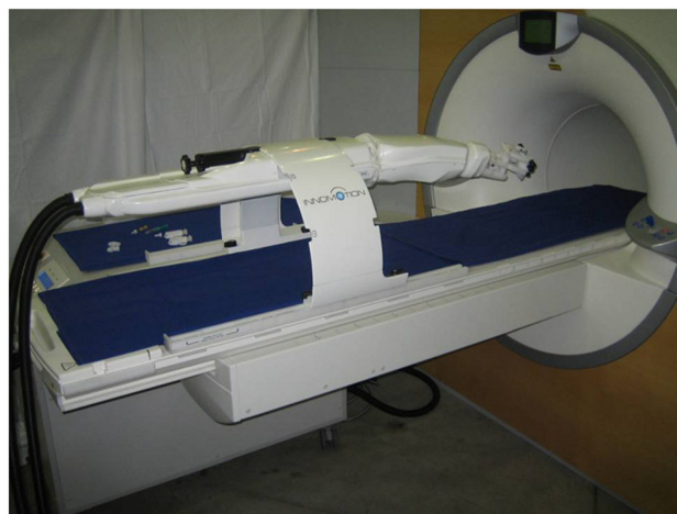
Figure 8. Innomotion robot, used for CT- and MR-guided needle-based procedures. Reprinted with permission from Innomedic GmbH. Copyright © Innomedic GmbH
