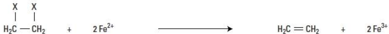
Figure 3.31. Example of a reductive transformation: electron transfer from \text{Fe}^{2+} to 1,2-dihalogen substituted ethane (X denotes a halogen atom).
