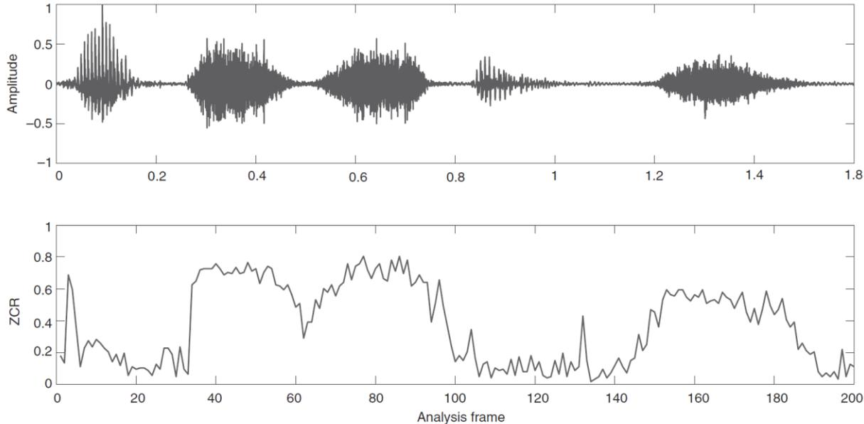
**Figure 7.2** The upper graph shows a recording of a male speaker saying ‘it’s speech’, which contains several stressed high-frequency sibilants and the lower graph is the frame-by-frame ZCR corresponding to this. The excursions of the ZCR plot closely match the high-frequency speech components, namely a breathy /i/ at the start, both /s/ sounds and the final /ch/.
