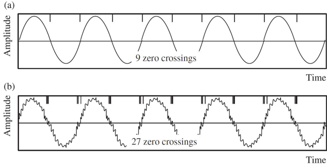
**Figure 7.1** Zero-crossing rate calculation illustrated for a pure sine wave (a) and one corrupted with noise (b). Zero crossings are indicated by tick marks at the top of each plot. The noise-corrupted sine wave below exhibits many more spurious zero crossings due to additive noise taking the signal backwards and forwards over the trigger amplitude several times each period.
