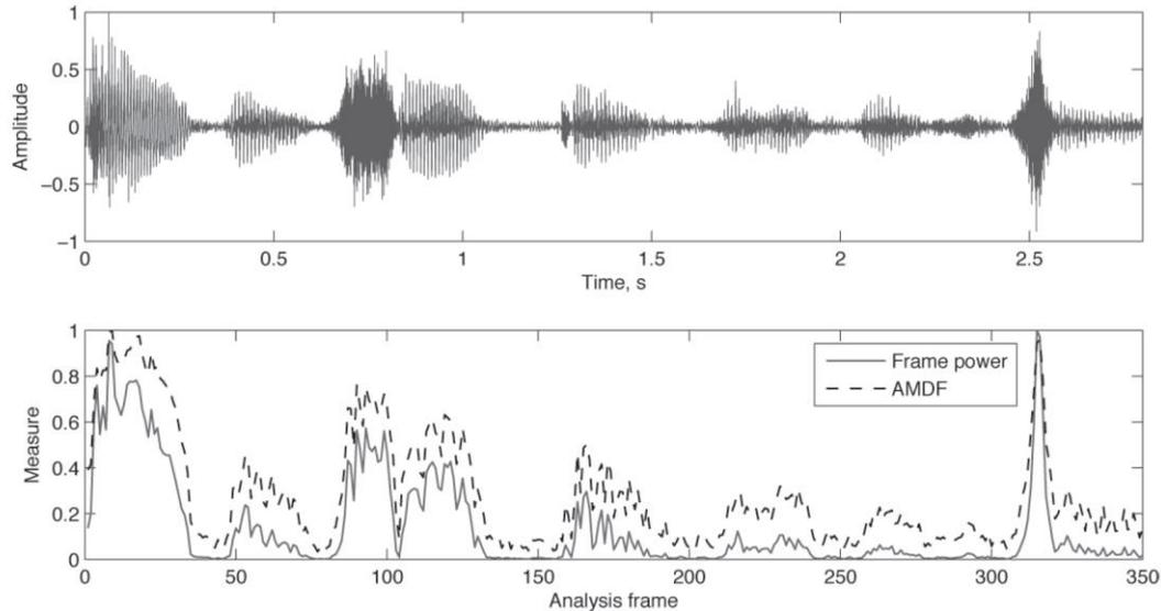
**Figure 7.4** Average magnitude difference function (AMDF) and frame power plots (lower graph) for a recitation of the alphabet from A to G (plotted as a waveform on the upper graph). The duration of the letter C is enough for there to be almost two amplitude ‘bumps’ for the /c/ and the /ee/ sounds separated by a short gap, spanning the time period from approximately 0.7 to 1.2 seconds.
