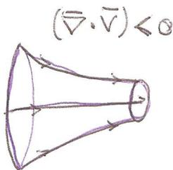
$$\frac{d\bar{\omega}}{dt} = -\bar{\omega} (\nabla \cdot \bar{v})$$
