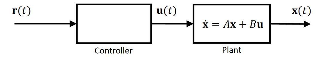
Given a reference trajectory r(t), design u(t) such that x(t) closely follows r(t)
