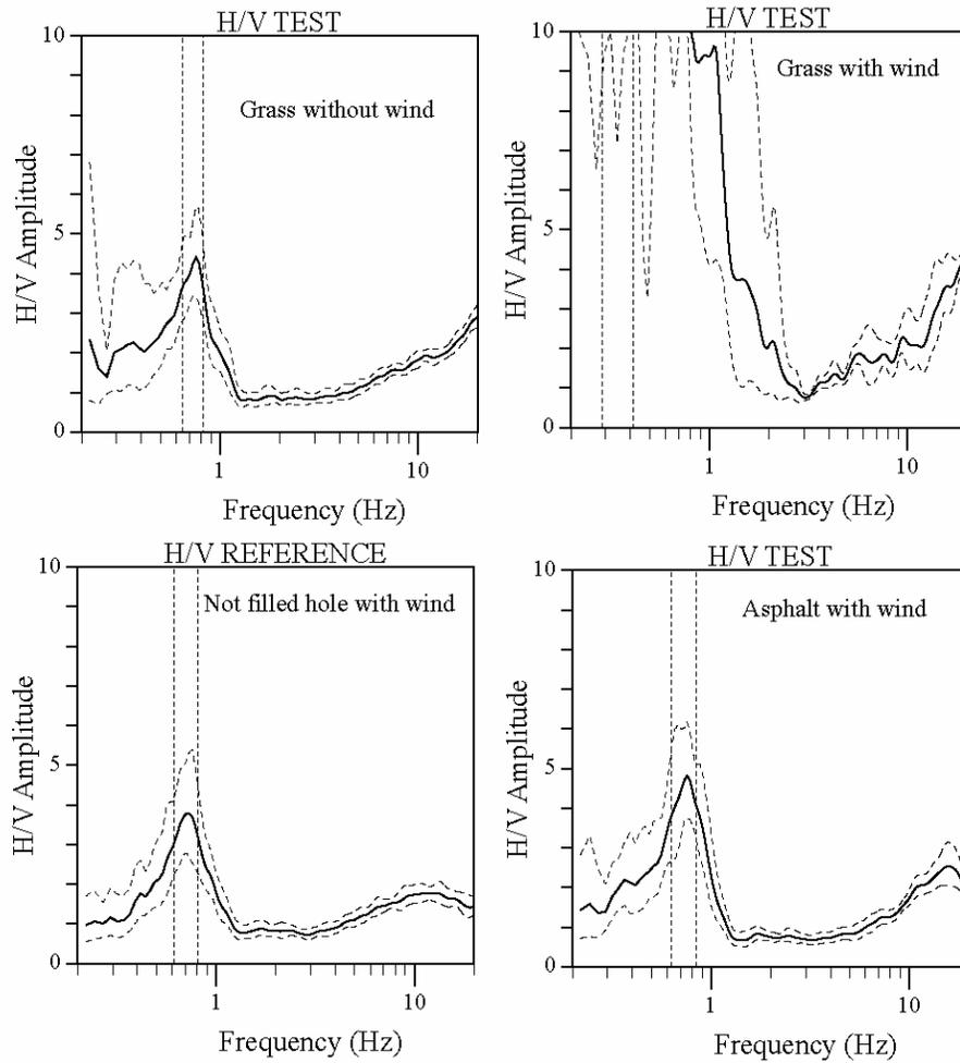
**Figure 2.** Comparison of the H/V curves obtained at the same site on grass with and without wind (top), and in a hole, on asphalt (bottom) and again on grass with wind. This comparison shows the strong effect of the wind combined with grass, whereas on asphalt or in a hole, the wind has no significant effect (if far away from any structure).
