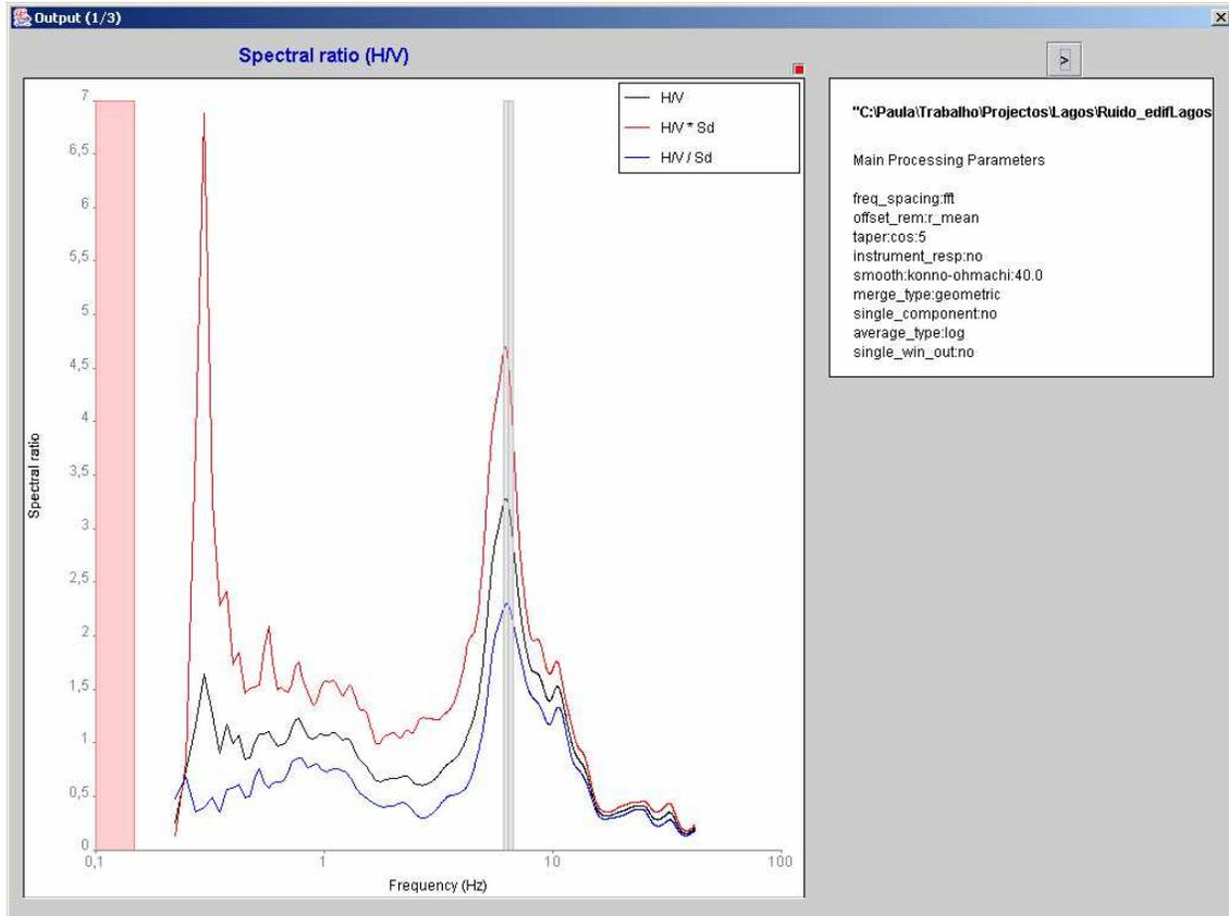
**Figure 6.** H/V ratio for the merged horizontal components (mean in black, mean multiplied and divided by  $10^{\sigma(\log H/V)}$ , in red and blue). The pink strip shows the frequency range where the data has no significance, due to the sampling rate and the window length. The grey strip represents the mean  $f_0$ , plus and minus the standard deviation. It is calculated from the  $f_0$  of each individual window.
