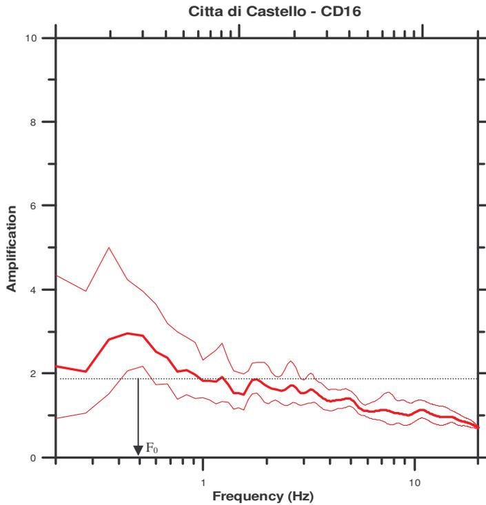
**Basin geometry:** Elliptical alluvium valley, width~10km, length~25km, depth~0.1km
