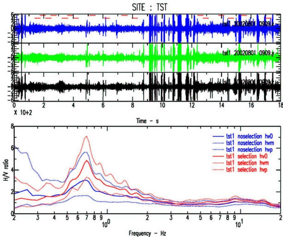
**Figure 5.** Signal (top) processed with (red curves bottom) or without (blue curves bottom) the automatic window selection (selected windows are indicated by the red segments on the top of the signal). The peak on the H/V curve is much clearer when the transient removal is applied, and also the standard deviation is lower, especially at low frequencies.
