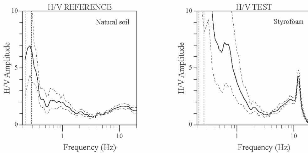
**Figure 3.** Comparison of the H/V curves obtained with and without a Styrofoam plate under the sensor, at the same site, showing a strong effect of the Styrofoam.
